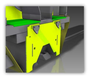
Typical DIN plate with the optional 6 pins for mounting on the truck:
